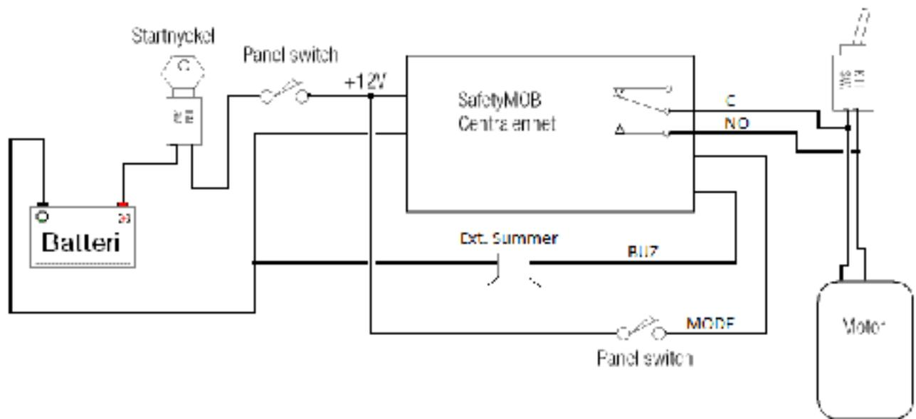
Installation in a boat with a short-circuit kill switch system.
