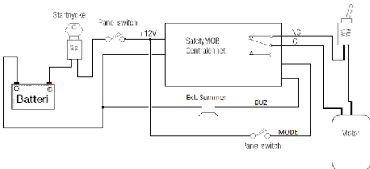
Installation in a boat with a breaking-up kill switch system.
